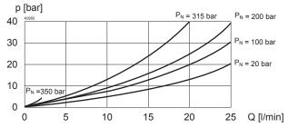
Q = f (p) Leakage volume flow characteristics
