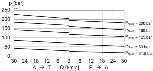
$p_{\text{red}} = f(Q)$  Pressure volume flow characteristics
