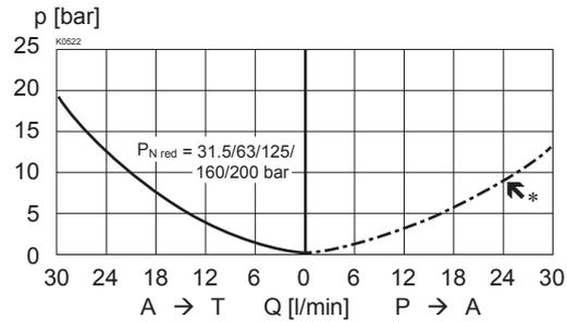
$p_{\text{red}} = f(n)$  Pressure adjustment characteristics
