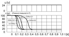
Schifting times, Influence of orifices on shifting Mesured with AMW4D101-G24, Q = 25 l/min Solenoid deenergised
