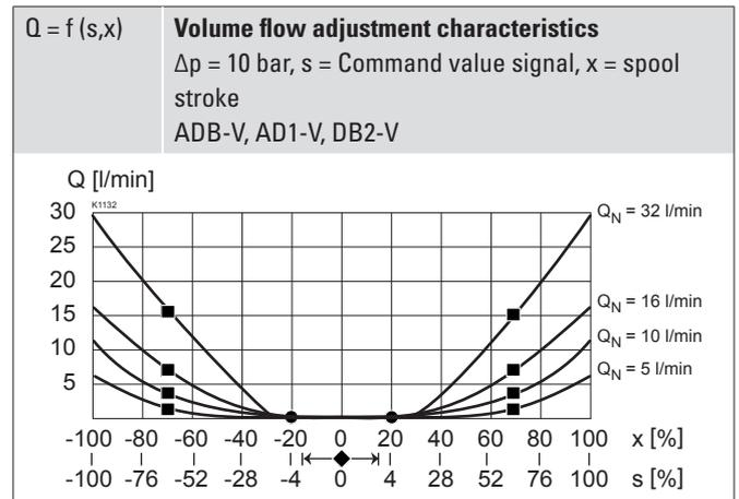
**Note!** All values were measured over two control edges. The connections A and B were short-circuited.
