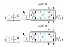
The middle position (a\*) is reached when the solenoid is only switched with 50 % power
