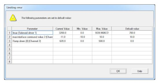
Parameter: Name of the parameter with the limiting value error
