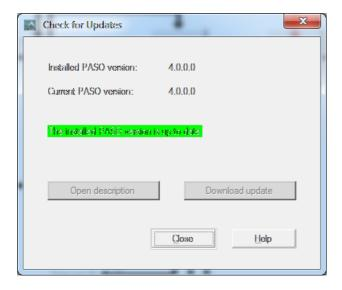
Next to "Installed PASO version", the version number of the installed PASO on the corresponding PC appears. Next to "Current PASO version", the version number of the newest PASO version appears.
