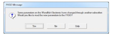
If the answer is "Yes", then the parameters will be read-in from the Wandfluh-Electronics. Possible open parameter windows in the PASO will be closed automatically. If a parameter value will be changed through the manual operation terminal after the read-in of the new parameters, this message will appear again.
