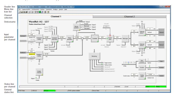
During the start-up, the parameterisation software PASO checks, whether a Wandfluh-Electronics device is connected. If no communication can be established, an error message appears (refer to section "Communication interruption" and the "Off Line"-mode will become active. All menu points and keys, which involve an action in connection with the communication, are then blocked. All other functions of the parameterisation software PASO can be utilised without any limitation.
