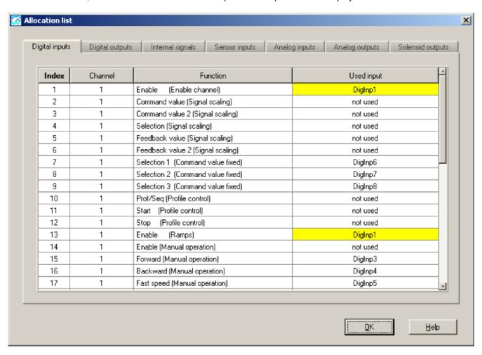
The display of the allocation list can be divided in digital inputs, digital outputs, internal signals, sensor inputs (only Enhanced controller version), analog inputs, analog outputs (only Enhanced version)and solenoid outputs. The display can be individually sorted (mouse click on the title bar of the desired column). Inputs and outputs which are double occupied have a yellow background (refer to section "Assignment of the inputs/outputs" [46]).
