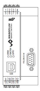
1 = Digital input 1 2 = Digital input 2 3 = Digital output 1 4 = Digital output 2 5 = Supply Analogue input + 6 = Supply voltage 0 VDC 7 = Stabilised output voltage 8 = Analogue ground 9 = Analogue input 1 + 10 = Analogue input 1 -11 = Analogue input 2 + 12 = Analogue input 2 -13 = Output solenoid 2 + 14 = Output solenoid 2 -15 = Output solenoid 1 + 16 = Output solenoid 1 -
