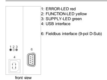
Front panel Basic-amplifier with HART interface:
