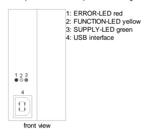
Front panel Enhanced-amplifier with CANopen/J1939 or Profibus DP interface:
