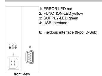
Front panel Enhanced-amplifier with HART interface:
