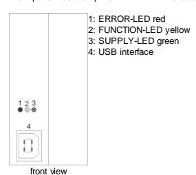
Front panel Enhanced-amplifier with analog interface:
