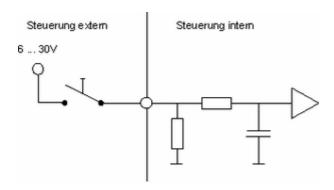
• The digital outputs are "Lowside Switch" outputs (open collector)
