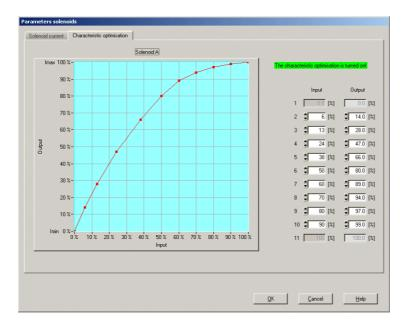
The solenoid current values are in the range lmin (0%) up to lmax (100%). Imin and lmax are adjusted in the menu "Solenoid current". At an input value which is between two graphic points, the solenoid current is interpolated. If two or more preset values overlap, at the corresponding Preset value the highest current value is calculated.
