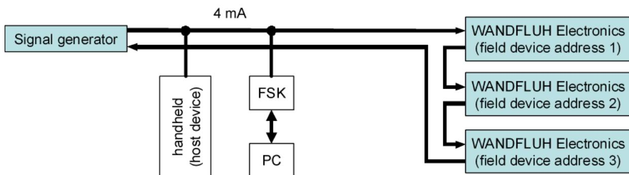
The HART protocol specifies the total load of the current loop (including the cable resistance) to be between minimum 230 Ohm and maximum 1100 Ohm. The burden on each WANDFLUH HART device is 250 Ohm. Therefore, a maximum of four WANDFLUH HART devices can be connected ( $1100 \text{ Ohm} / 250 \text{ Ohm} = 4$ ).
