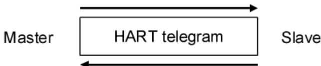
In the section [Telegram structure](#)<sup>[9]</sup> there is a description about the whole HART transfer available. For the transfer of the HART commands, only bytes CD, BC, Status and Data are used.
