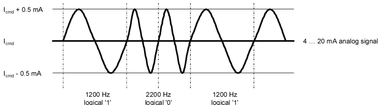
To encode the bits, the FSK method (Frequency Shift Keying) based on the Bell 202 communication standard is used. Thereby, the following frequencies are used:
