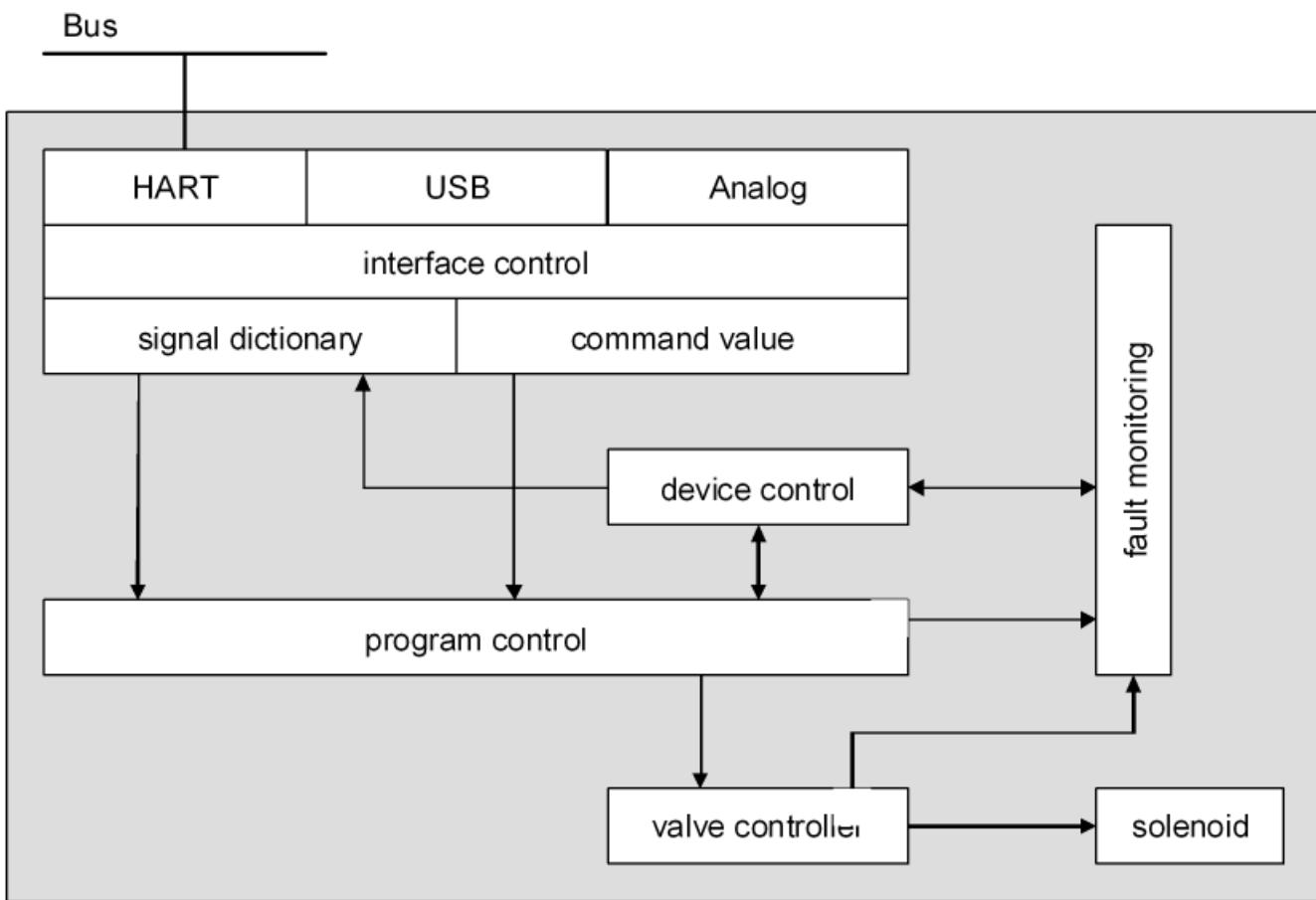
The HART field device contains the complete Hardware of the *WANDFLUH-Electronics*. This Hardware includes the interface for the Fieldbus and the interface for the parameterisation software PASO. Also included are the solenoid outputs.
