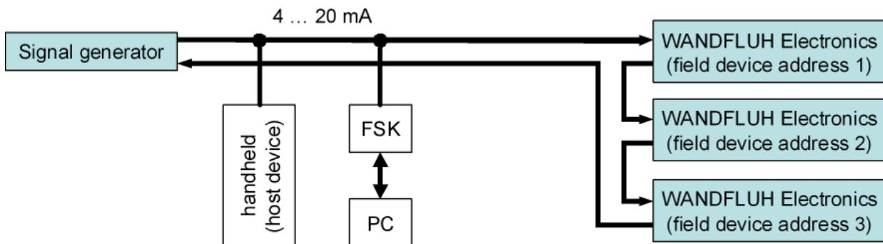
The HART protocol specifies the total load of the current loop (including the cable resistance) to be between minimum 230 Ohm and maximum 1100 Ohm. The burden on each WANDFLUH HART device is 250 Ohm. Therefore, a maximum of four WANDFLUH HART devices can be connected (1100 Ohm / 250 Ohm = 4).
