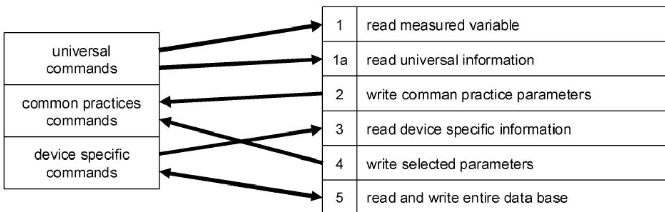
Depending on the tasks to be executed, the HART master device uses a command that can be assigned to one of the six different conformance classes. Each conformance class contains a subset of HART commands which cover a special administrative or control-related range of tasks.
