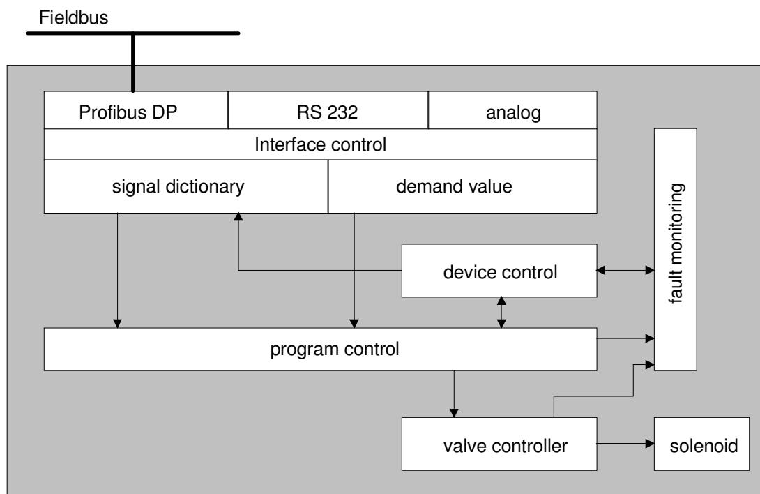
The DP-Slave controller card contains the complete Hardware of the SD6 Electronics. This Hardware includes the interface for the Fieldbus and the interface for the parameterisation software PASO. Also included are 2 solenoid outputs for the cylinder.
